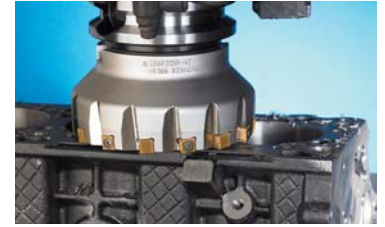
Roughing for cast iron
